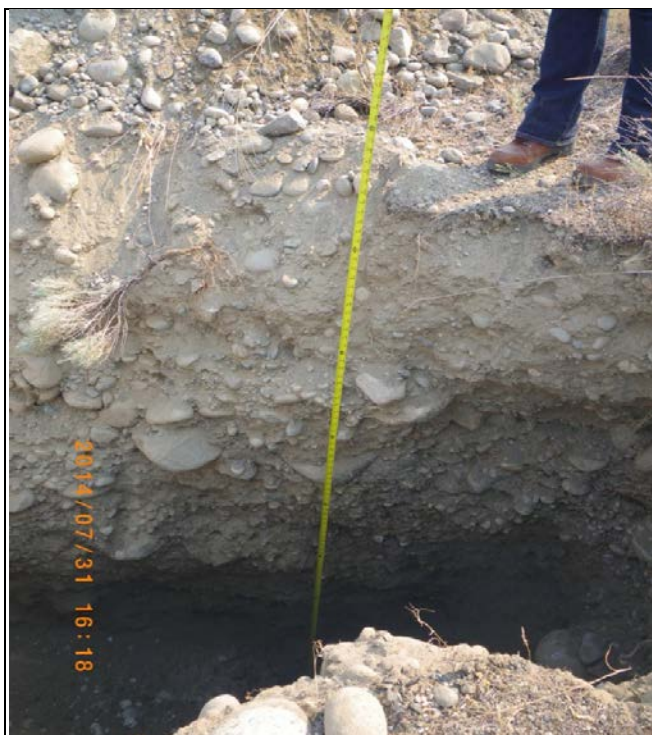
Figure 14. Excavation of 14-BH-11 to bottom of thrust at 4.5 feet below ground surface. Gravels, sand; no cultural clasts. Location adjacent to former course of Foster Creek suggests that deposit is torrential fluvial (bed load) in origin.
