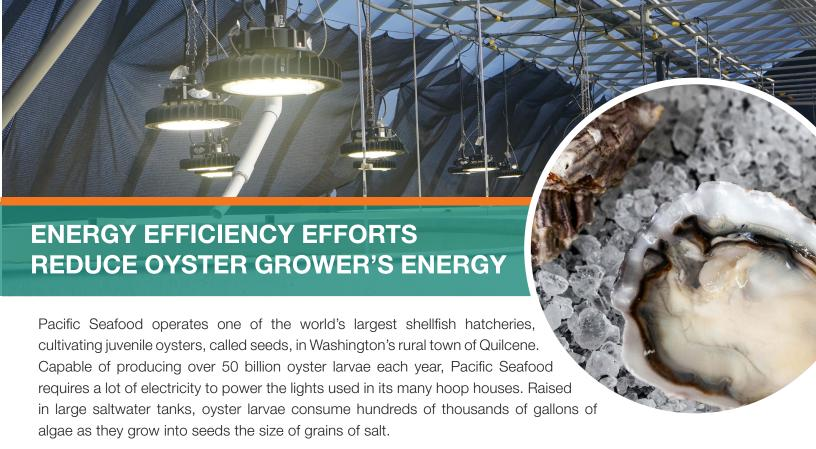
Earlier this year, Jefferson County PUD saw an opportunity to aid Pacific Seafood with lighting upgrades. Replacing the large metal 1,000-watt halide bulbs with energy-efficient 250-watt LEDs has led to a 75% reduction in the company's Quilcene facility power consumption for lighting. The project used the utility's Energy Efficiency Incentive fund, provided by the Bonneville Power Administration.
