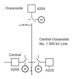
The Dispatcher will contact a Switchman at each terminal and request the reclosing relays cutout on PCBs 4209 and 4220 at Central Substation and on PCB 4204 at Oceanside Substation, and the reclosing relays and each PCB control switch be tagged with a Hold Order for the Dispatcher.
