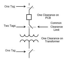
If two Clearances are issued on the PCB and one Clearance on the transformer bank, two Do Not Operate tags would be hung on the common Clearance limit. The other disconnect switches would each have one Do Not Operate tag hung on them. (Refer to the following drawing).
