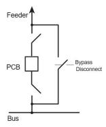
The Switchman would tag the open hot-stick operated Bus Disconnect and Feeder Disconnect with red Do Not Operate tags which are attached to red wooden blocks and checked "See Tag in the PCB control cabinet".
