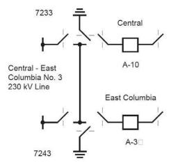
Normal Dispatching/SCADA operating procedures would de-energize the Central-East Columbia No. 3 230 kV line by opening PCBs A-10 and A-3 by supervisory control.
