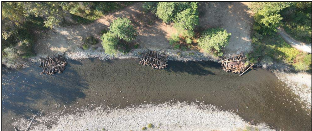
Figure 4: 2022020(Suspension Reach)LW bank buried structure
