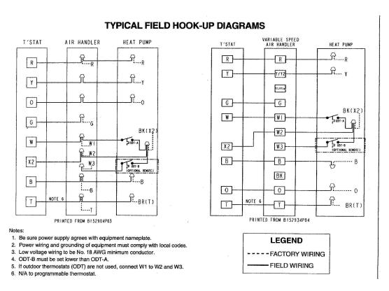
Before installation is considered complete, confirm the emergency heat circuit energizes the strips. Also, as part of this installation, make sure the auxiliary and emergency heat circuits are controlled separately; if they are not, a different thermostat or other wiring work-around will be needed.
