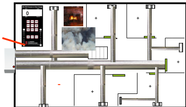
House Pressures Resulting from Closed Interior Doors
