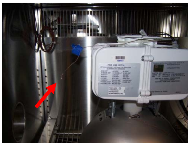
Figure 20: Thermocouple monitoring temperature inside test chamber
