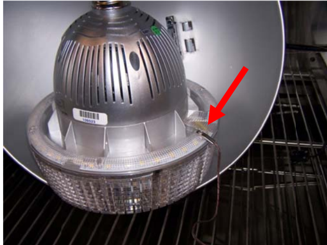
Figure 18: Thermocouple attached to the lamp
