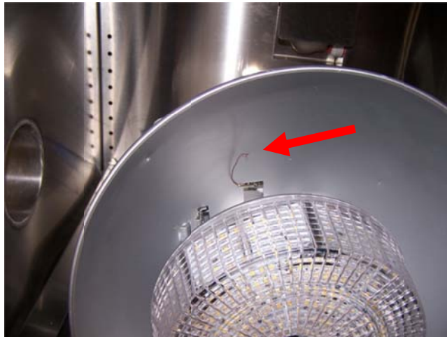
Figure 19: Thermocouple monitoring temperature inside the luminaire
