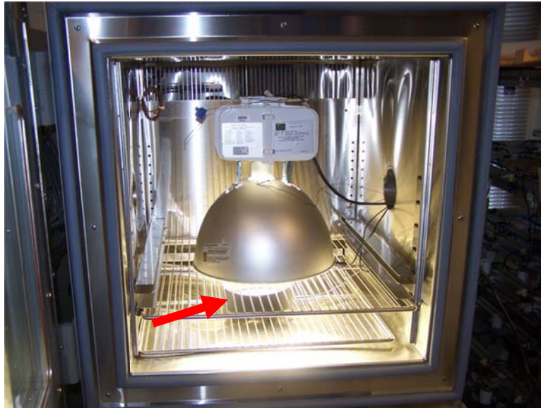
Figure 21: Photodiode located on rack below luminaire monitoring luminaire light output
