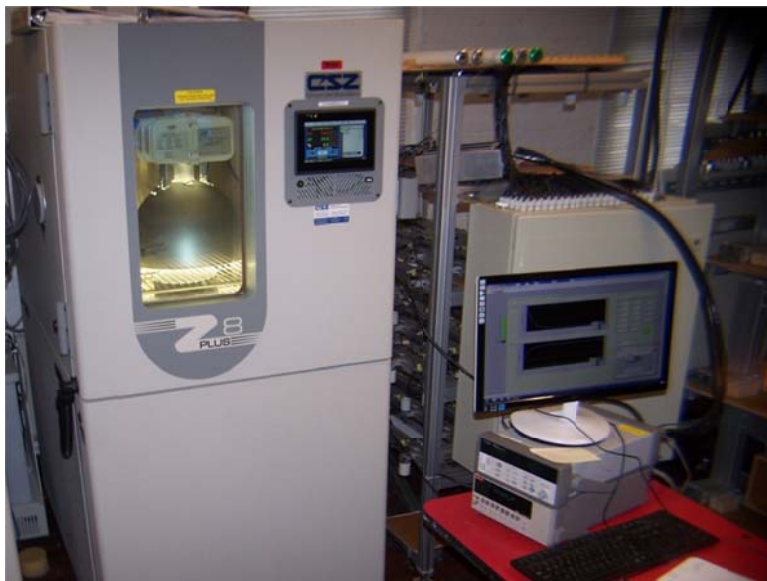
Figure 17: CSZ Test Chamber and computer monitoring setup. Luminaire energized inside the test chamber is the tested high bay luminaire.
