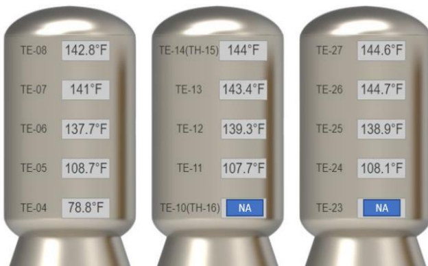
Figure 12. Snapshot of temperatures in thermal storage system
