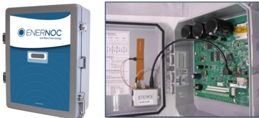
Figure 8: EnerNOC Site Server
