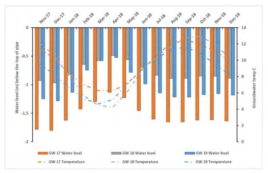
Figure 12. Longley Meadows reach monthly average groundwater levels for Wells 17-19 and corresponding groundwater temperatures. November 2017 to December 2018; colors for groundwater temperatures and levels are matching.
