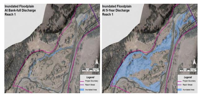
Figure 2. Floodplain inundation at bankfull discharge (left), and at 5-year recurrence interval (right).
