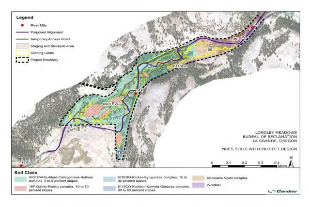
Figure 22. Active project area showing proposed project elements and mapped soil units based on the Soil Survey Report of Union County Area (2018).
