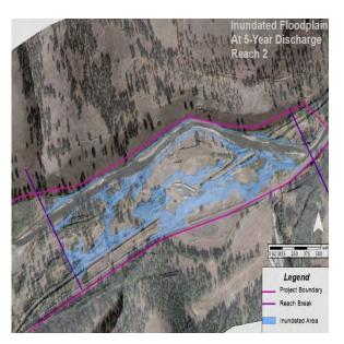
Figure 19. Floodplain inundation at 2-year recurrence interval (left) and at 5-year recurrence interval (right).
