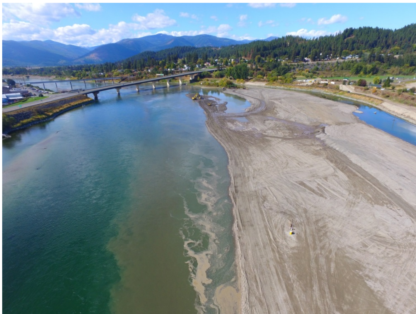
Figure 11. Sediment plume during 2015 Island Construction
