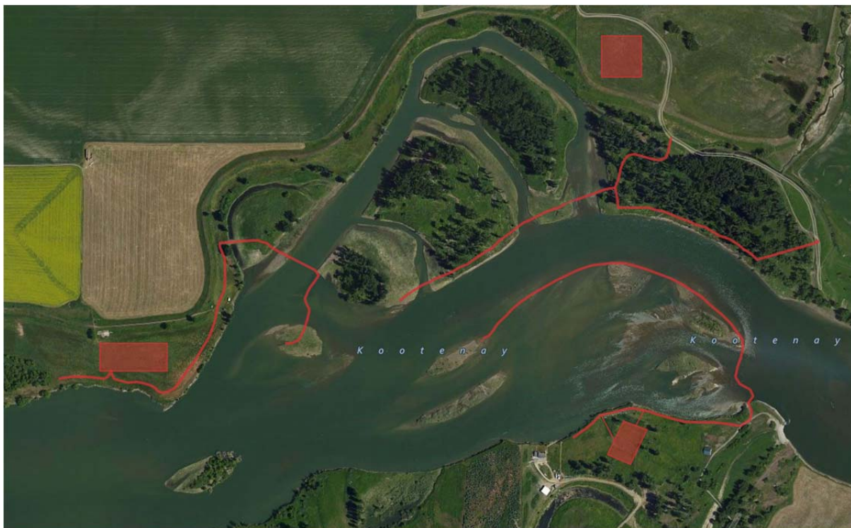
Figure 8. Staging areas and temporary haul roads
