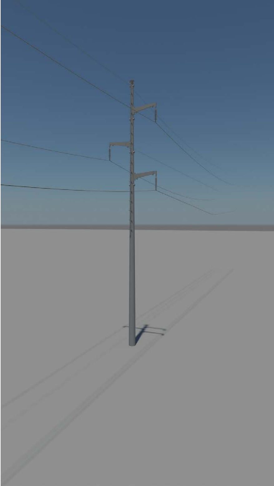
Figure B-2. 3-D Model of Single-circuit Steel Pole Structure Used for Photographic Simulations
