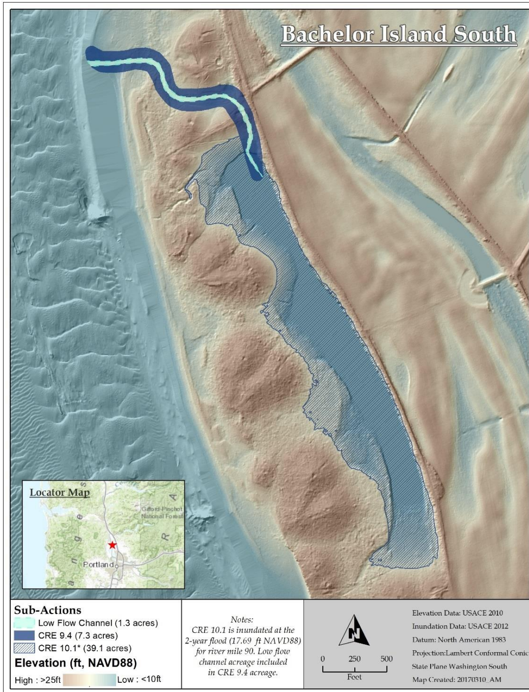
Figure 5: Elevation map of proposed channel construction and the action area, with layers added by the type of restoration action expected as outlined in NMFS' 2011 Columbia River Estuary Module.
